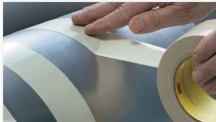
3M™ Traction Tape 5401 enhances friction on web rollers to help maintain constant traction and tension for the web material from start-up through wind-up.
