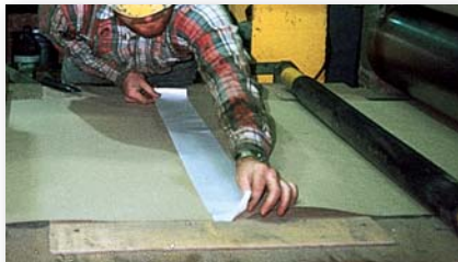
With high tensile strength and rubber adhesive, 3M™ Glass Cloth Tape 365 reliably splices fabrics and other textured surfaces.
